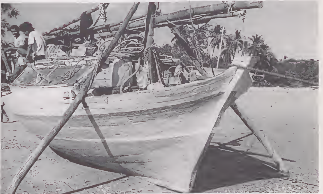
Fig. 15. A small sope type boat with a light stem at Namu Sain near Kupang, Timor.
